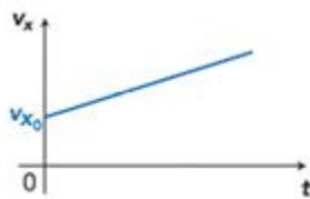
$$v_x(t) = \frac{dx}{dt} = a \cdot t + v_{x0}$$
